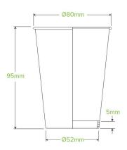
Aqueous Single Wall BioCups are manufactured using a unique water-based dispersion coating certified home compostable to European standards (NF T51-800 ). These cups are food safe, odorless, and can be disposed of right in your backyard compost bin!
