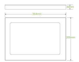
BioBoard catering tray lid is made from FSC™ certified paperboard. The windowed lid is made from a bioplastic made from plants, not oil, and is certified industrially compostable.
