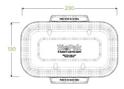
Our plastic-free sugarcane takeaway container lids are made from rapidly renewable sugarcane pulp, a by-product of the sugar refining industry. These 750 & 1,000ml white bagasse food container lids are microwave and oven safe.
