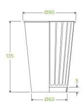
Paper BioCups are made from premium paperboard lined with a plant-based bioplastic. These eco-friendly disposable cups are certified industrially compostable. This 16oz Leaf double wall cup fits our large lids.
